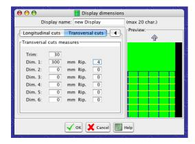
The operators inputs cutting measures aided by a comfortable preview that show the cutting position as well as entered.
